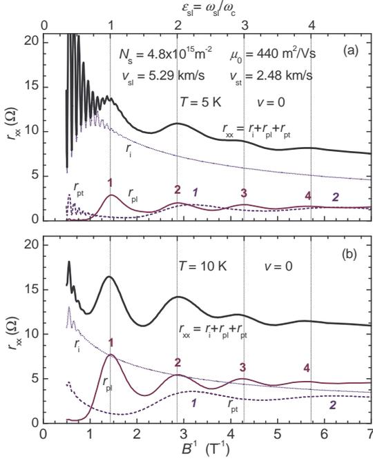
FIG. 1: (Color online) Linear ( $v = 0$ ) resistivities ( $r_{xx}$ ,  $r_i$ ,  $r_{pl}$ , and  $r_{pt}$ ) at (a)  $T = 5$  K (a) and (b)  $T = 10$  K for a GaAs-based heterosystem with carrier sheet density  $N_s = 4.8 \times 10^{15} \text{m}^{-2}$  and zero-temperature linear mobility  $\mu_0 = 440 \text{m}^2/\text{Vs}$ . The longitudinal and transverse sound velocities are taken to be  $v_{sl} = 5.29 \times 10^3 \text{m/s}$  and  $v_{st} = 2.48 \times 10^3 \text{m/s}$ .
