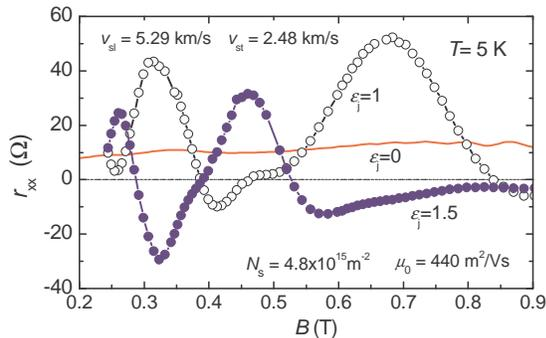
FIG. 4: (Color online) Differential resistivity  $r_{xx}$  is plotted versus magnetic field  $B$  for fixed values of  $\varepsilon_j = 0, 1,$  and  $1.5$  at  $T = 5$  K.
