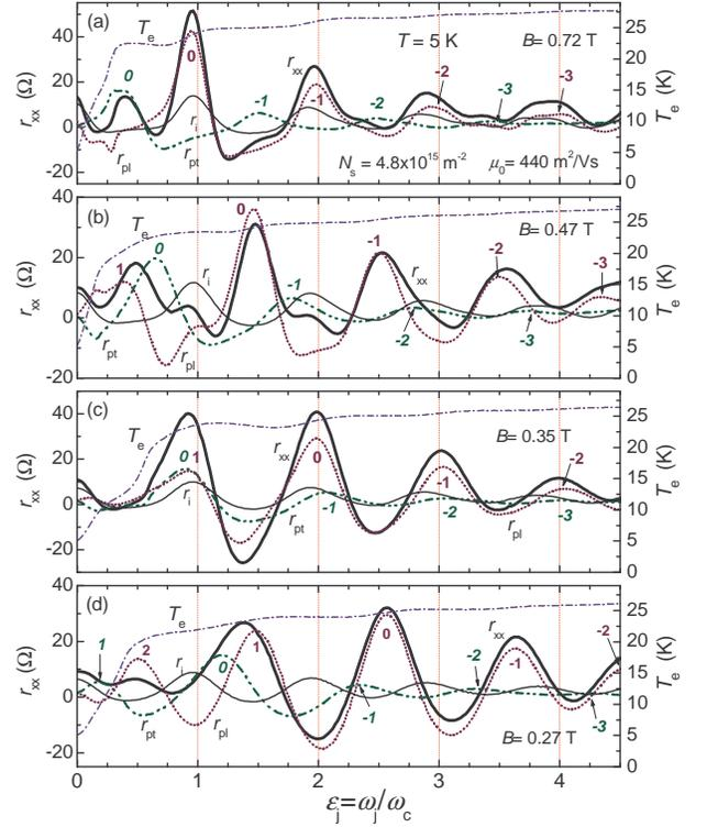
FIG. 3: (Color online) Differential resistivities ( $r_i$ ,  $r_{pt}$ ,  $r_{px}$ , and  $r_{xx}$ ) and electron temperature  $T_e$  are shown as functions of  $\varepsilon_j$  at fixed magnetic fields  $B = 0.27, 0.35, 0.47$ , and  $0.72$  T, respectively, at  $T = 5$  K. The number near the peak of  $r_{pt}$  or  $r_{px}$  is the value of the integer  $l$  in the resonance condition (19) of the corresponding differential resistivity peak.
