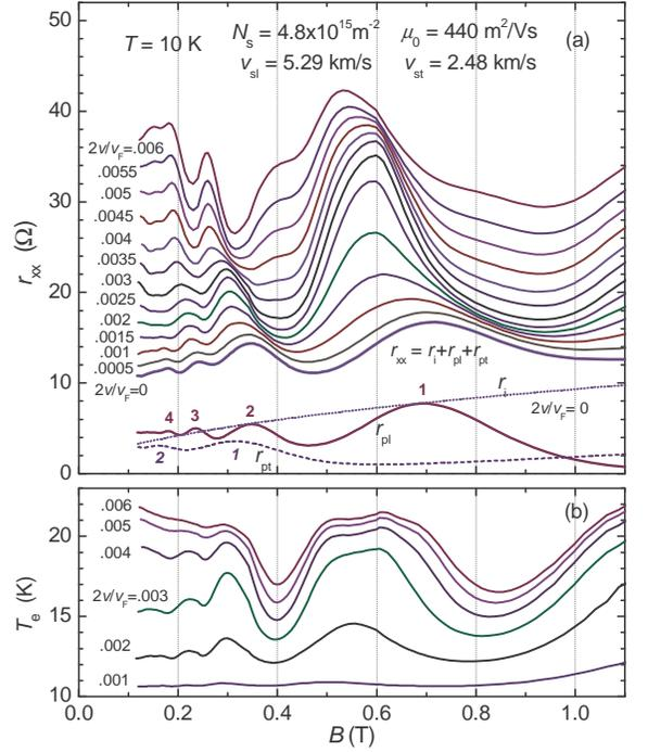
FIG. 2: (Color online) (a) Differential resistivities  $r_{xx}$  and (b) electron temperature  $T_e$  are shown as functions of the magnetic-field strength  $B$  at lattice temperature  $T = 10$  K under different values of the bias drift velocity  $v/v_F$ . Here,  $v_F$  is the Fermi velocity of the 2D electron system, and  $r_{xx}$  curves of different  $2v/v_F$  values are vertically offset for clarity.
