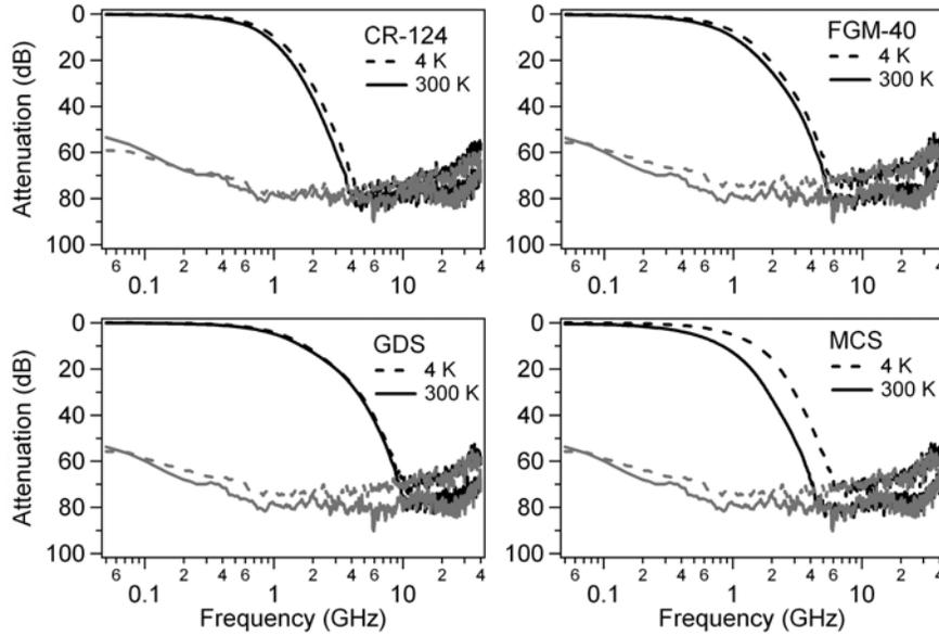
**Figure 2.** Measured attenuation of the CR-124, FGM-40, GDS, and MCS stripline filters at room temperature (solid line) and 4.2 K (dashed line). The instrument noise floor is indicated in grey. (The noise floor is higher at 4.2 K because of the loss of the extra cables used to measure at low temperature.)
