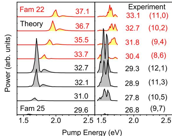
FIG. 3: (color online) Coherent phonon intensity at the RBM frequency as a function of pump/probe energy for several mod 2 semiconducting nanotubes at the  $E_{22}$  transition. Right: experimental spectra; left: simulated spectra. The upper four curves in each panel are for nanotubes in Family 22 and the lower four curves are for tubes in Family 25. Each curve is labeled with the chirality  $(n,m)$  and the RBM phonon energy in meV and offset for clarity.
