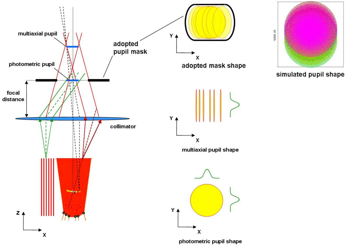
Fig. 3. Shape and location of the photometric and multi-axial pupils (left); shape of the adopted pupil mask to be placed at the collimator focal distance (center); ZEMAX simulation of the pupil shape (right).
