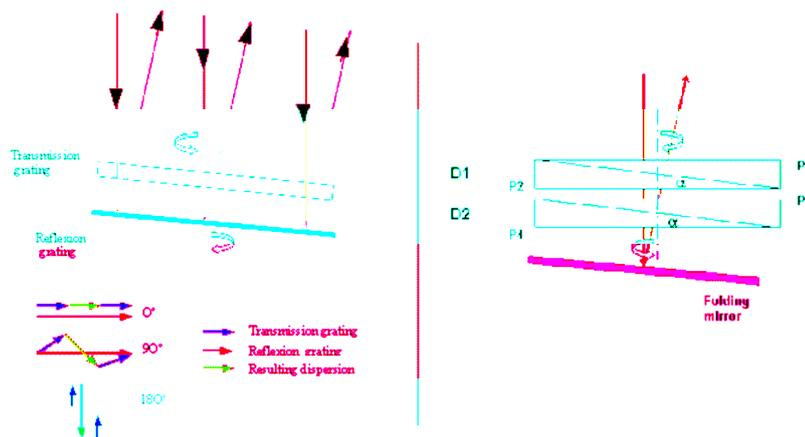
Fig. 9. Concept of the low resolution dispersers.
