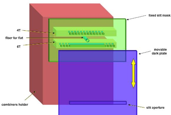
Fig. 8. Cold plate device for both slit mask and dark.
