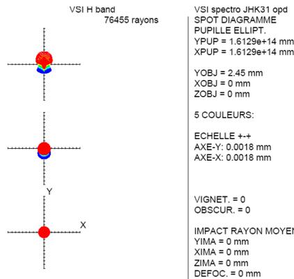
Fig. 7. Spot diagram (cross size is 36 $\mu$ m).
