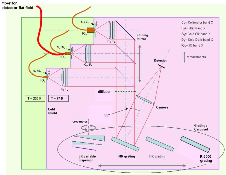
Fig. 1. Sketch of the overall spectrograph layout. Each beam combiner has its own optimized collimator.
