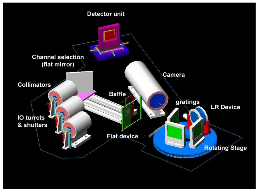
Fig. 10. 3D overall layout of the mechanical assembly of the spectrograph.
