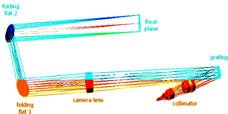
Fig. 6. VSI Spectrograph optical layout.
