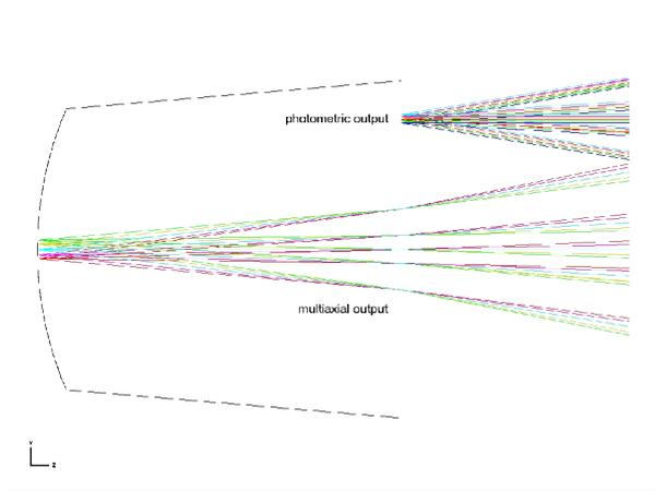
Fig. 4. ZEMAX simulation of the light cones exiting out of the 6T combiner (top view).
