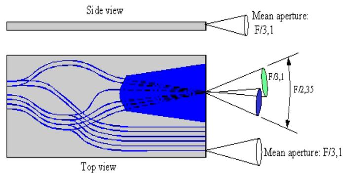
Fig. 2. Beam combiner output features.
