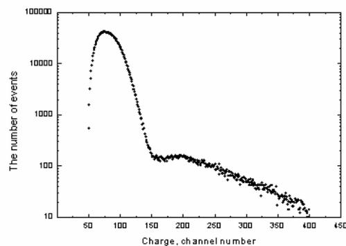
Fig.3. Charge spectrum of the events detected with the scintillator counter at the underground laboratory at the depth of 200 m.w.e..
