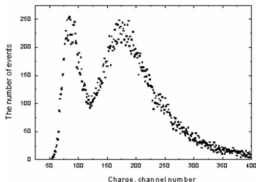
Fig.2. Charge spectrum of the events detected with the scintillator counter in the surface laboratory.
