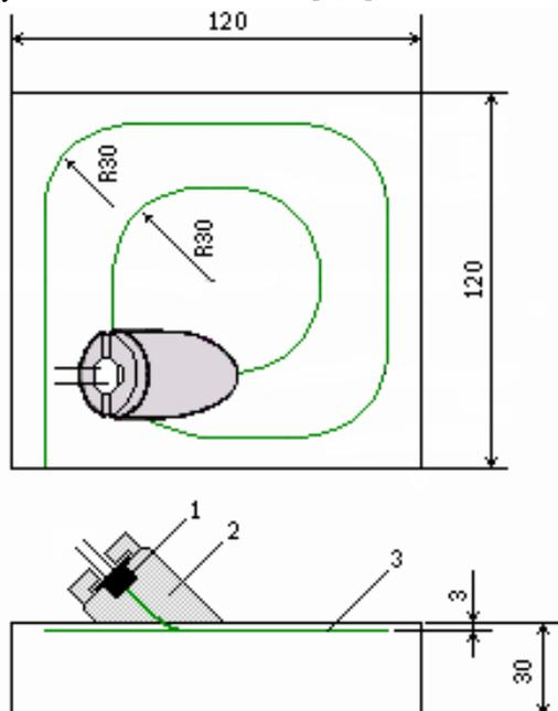
Fig.1. Schematic view of the scintillator counter. 1 – MRS APD; 2 – connector; 3 – WLS fibre.
