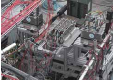
Figure 10: The microMegas digital HCAL prototype in the beam line at CERN in summer 2008.
