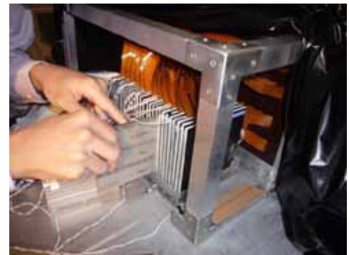
Figure 4: Scintillator Tungsten ECAL prototype.
