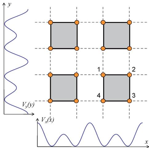
FIG. 1: (Color online) The optical superlattice consists of a periodic array of  $2 \times 2$  plaquettes. The 2D optical trapping potential is created by adding two superlattice potentials  $V_x(x)$  and  $V_y(y)$  illustrated in the bottom and left panels. The intra-plaquette coupling is represented by the solid lines and the inter-plaquette coupling is represented by the dashed lines.
