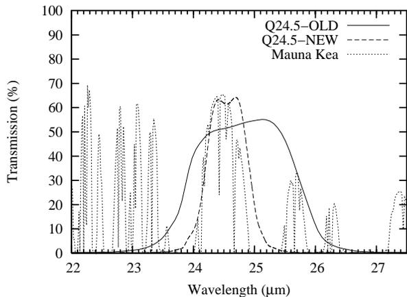
**Fig. 1.** Transmission curves for the Q24.5-OLD filter (solid line), Q24.5-NEW (dashed line), and the atmosphere above Mauna Kea (dotted line). The filter transmission spectra have been made available by the manufacturer. The atmospheric transmission curve has been calculated using USF HITRAN-PC for a standard ‘US tropical model’ with an  $\text{H}_2\text{O}$  partial pressure of 1.35 mmHg at 4200 m looking through the atmosphere at a zenith angle of  $30^\circ$  (Tomono 2000).
