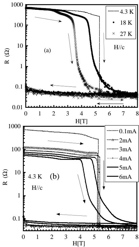
FIG. 2: (a)  $ab$ -plane magnetoresistance data of the  $z=0.6$  crystal at selected temperatures of 4.3, 18 and 27 K for  $I=0.1\text{mA}$ . ( $H||c$ ) (b)  $ab$ -plane MR data as a function of an applied current from 0.1 up to 6 mA.
