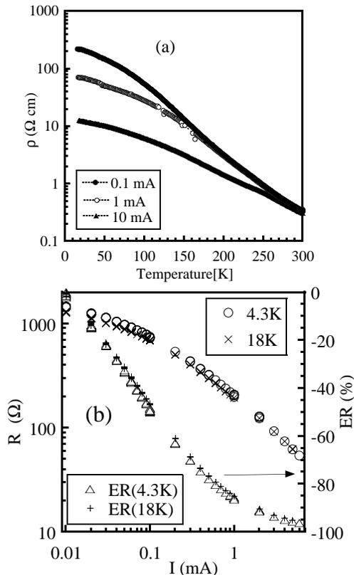
FIG. 1: (a) The temperature variation of  $ab$ -plane resistance of the  $z=0.6$  crystal measured for various applied currents of 0.1, 1 and 10 mA. (b) The electroresistance (ER) and the ER ratio on the  $ab$  plane at lower temperatures of both 4.3 and 18 K up to 6 mA.
