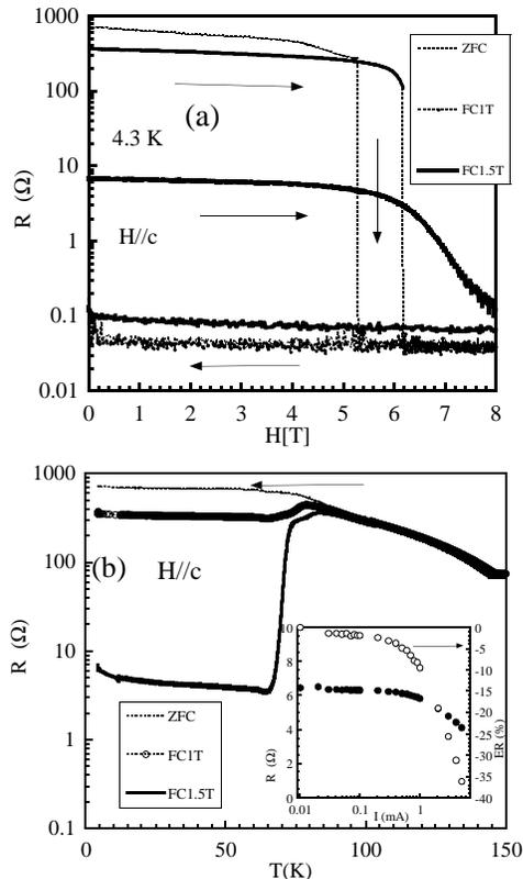
FIG. 3: (a)  $ab$ -plane MR data of the  $z=0.6$  crystal after the field cooling (FC) runs, FC-1T and FC-1.5 T, at  $I = 0.1$  mA ( $H||c$ ). For comparison, the zero-field cooling (ZFC) data are presented. (b) the temperature profile of the resistance monitored in the FC process from 150 K down to 4 K. The inset presents the ER and the ER ratio in the FC-1.5 T case at 4.3 K.
