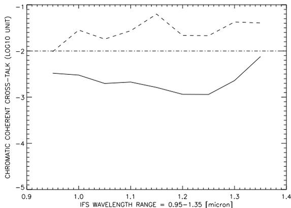
FIG. 15.— Coherent cross-talk coefficient as a function of the wavelength in the range  $0.95 - 1.35 \mu\text{m}$ . Solid line represents the BIGRE solution, dashed line the TIGER one and dot-dashed line the SPHERE IFS specification.
