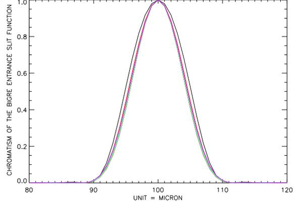
FIG. 9.— Normalized BIGRE entrance slit function: the example shows the case of the IFU optimized for SPHERE in the working wavelengths range:  $0.95 - 1.35 \mu m$ ; colors indicate seven distinct wavelengths.
