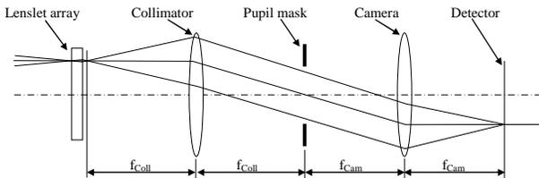
FIG. 12.— BIGRE spectrograph concept: the entrance slits plane is filled with the micro-images of the the first surfaces of the BIGRE spaxels and the spatial filtering is done in the metapupil plane forming between collimator, having focal length  $f_{Coll}$  and the re-imaging optics, having focal length  $f_{Cam} \equiv m_{IFS} \cdot f_{Coll}$ .
