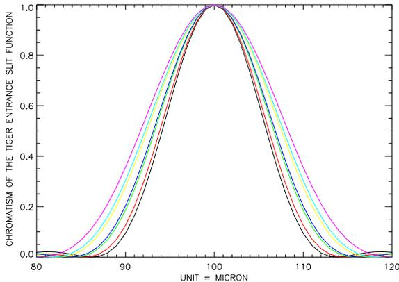
FIG. 7.— Normalized TIGER entrance slit function: the example shows the case of the IFU optimized for SPHERE in the working wavelengths range:  $0.95 - 1.35 \mu\text{m}$ ; colors indicate seven distinct wavelengths.
