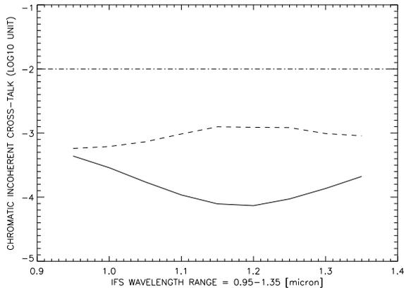
FIG. 14.— Incoherent cross-talk coefficient as a function of the wavelength in the range  $0.95 - 1.35 \mu\text{m}$ . Solid line represents the BIGRE solution, dashed line the TIGER one and dot-dashed line the SPHERE IFS specification.
