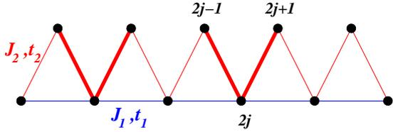
**Figure 1.** The sawtooth chain. The exchange (hopping) integrals are  $J_1$  ( $t_1$ ) along the base line and  $J_2$  ( $t_2$ ) along the zigzag line. The bold valleys show the area occupied by localized magnons (electrons).
