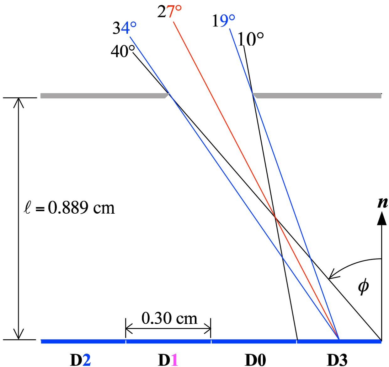
Fig. 1.— Sketch showing the detector-aperture geometry of STE-D in the ecliptic plane, also the mid-plane of the system (see Fig. 2 of Lin et al., 2008). Each of the four detectors has area  $.09 \text{ cm}^2$ . The aperture has dimensions  $0.3 \text{ cm}$  by  $1.22 \text{ cm}$ , oriented normal to the page. Detectors D2 and D3 each have geometrical factor  $0.021 \text{ cm}^2 \text{ sr}$ . The entire system has a geometrical factor  $0.10 \text{ cm}^2 \text{ sr}$  (Lin et al., 2008).
