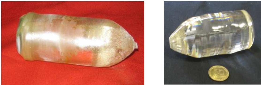
Fig. 1. CdWO<sub>4</sub> (mass 3 kg, left) and ZnWO<sub>4</sub> (≈1.3 kg, right) single crystals.
