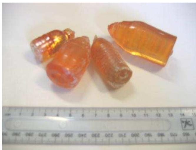
Fig. 6.  $\text{ZnMoO}_4$  single crystals.
