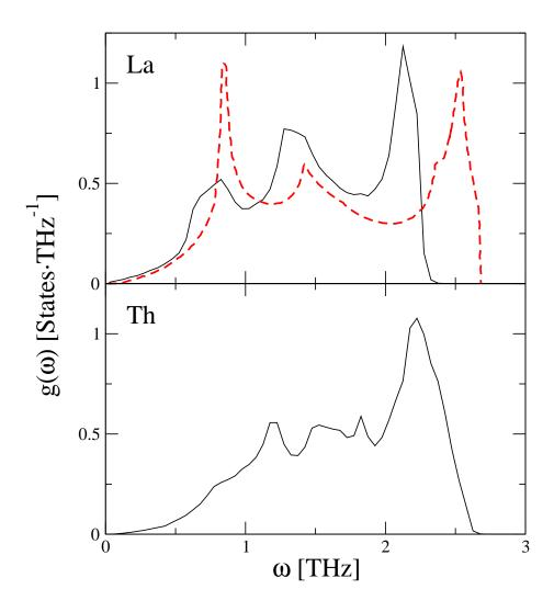
Figure 2. (color online) The phonon density of states for bcc La and bcc Th. The black curves are the 1163 K and 1636 K SCAILD calculations for La and Th, respectively. The dashed red line is the experimental bcc La data calculated from the 1163 K measurements of Güthoff et~al~[19]. Both the experimental and the theoretical density of states  $g(\omega)$  have been normalized so that  $\int_0^\infty g(\omega)d\omega=1$ .
