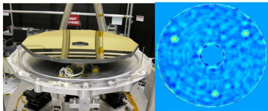
**Figure 8:** Actuated hybrid mirrors (AHM) of less than  $15 \text{ kg/m}^2$  have been tested and demonstrated  $40 \text{ nm}$  total WFE (gravity effect included), limited by high-spatial frequency mandrel polishing residual errors. With a higher quality mandrel,  $10 \text{ nm}$  surface figure error is achievable for meter-class segments.
