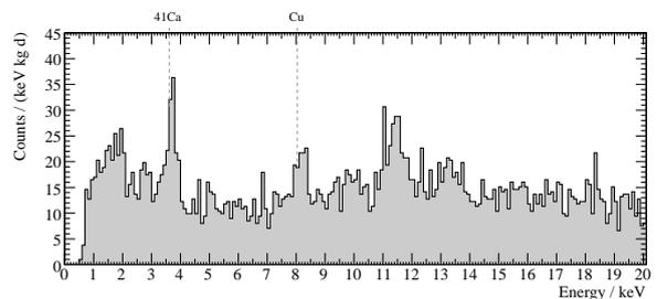
Figure 8: Low-energy part of the spectrum shown in figure 5. In addition to the lines from  $^{41}\text{Ca}$  and copper fluorescence there is a line at  $\sim 11.5 \text{ keV}$  which so far could not be identified in a consistent way (detector VERENA, run 30).
