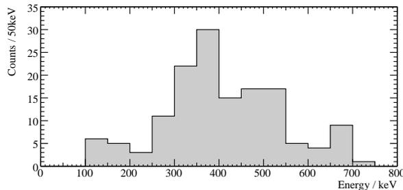
Figure 12: Histogram of all coincident events in one detector that appear at  $(307 \pm 3)$  keV in the respective other detector: The  $^{176}\text{Lu}$  beta spectrum starting at 290 keV is visible despite the low statistics.
