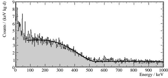
Figure 3: Background spectrum observed with one crystal ( $m = 306.8$  g) from an exposure to background radiation of 15.00 kg d early 2004 (detector DAISY, run 28). The black line is a fit above 80 keV of a parametrization of the <sup>90</sup>Sr/<sup>90</sup>Y beta spectrum to the data.
