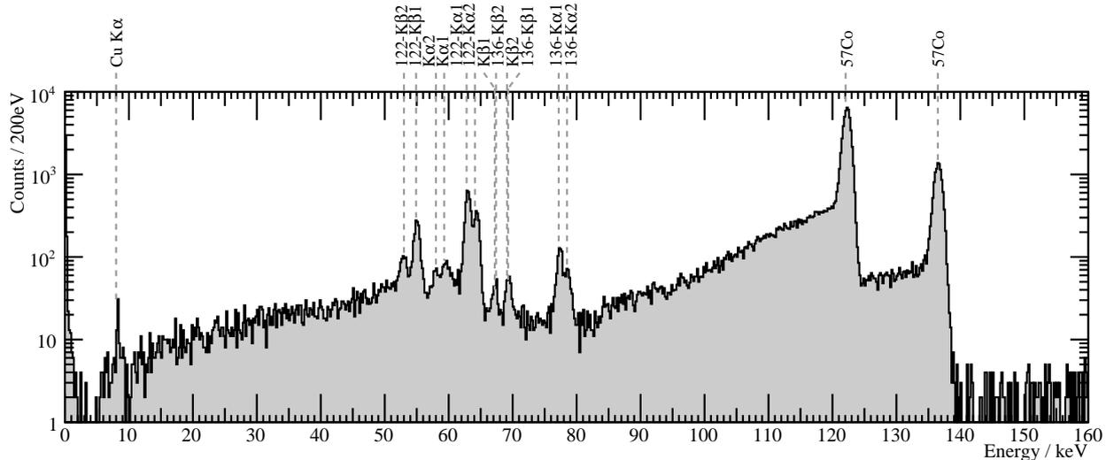
Figure 2: Energy spectrum from a high statistics  $^{57}\text{Co}$  calibration (detector DAISY, run 31).
