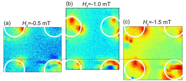
Fig. 2: Visualization of superconducting vortices pinned by Py dots at 6.1 K ( $72\%T_c$ ). For a better visualization of the vortex positions the “background” image was subtracted. The frozen effective fields  $\Delta H_z$  are: (a)  $-0.5$  mT, (b)  $-1$  mT and (c)  $-1.5$  mT. SC vortices are visualized as red spots.
