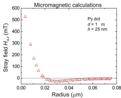
Fig. 4: Stray field distribution just above the surface of the Py dot in the vortex state. The estimated values are based on micromagnetic calculations using the LLG-program [19].
