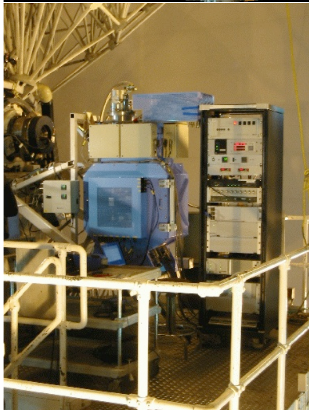
Figure 1. HARP shown on the right-hand Nasmyth platform of the JCMT, and a zoomed-in image of HARP and the instrument electronics box.
