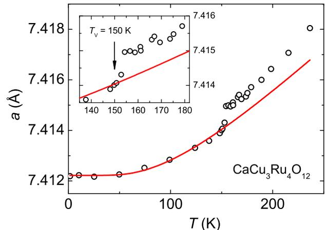
FIG. 1: Temperature dependence of the lattice constant  $a$  of  $CaCu_3Ru_4O_{12}$  as resulting from the Rietveld refinements of the neutron powder-diffraction measurements. The solid line is a fit according to an usual anharmonic behavior described in the text.
