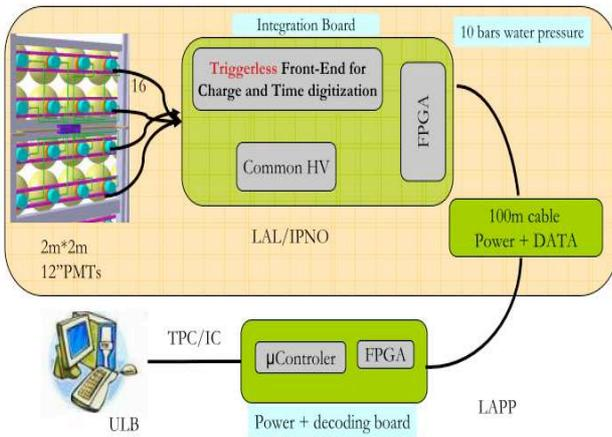
Fig. 2. Principle of the PMM<sup>2</sup> project. The main blocks are shown: the integration board that receive the PMT signal and transmit by 100 m of cable the 52 bits of DATA (for each channel) to the surface controller.
