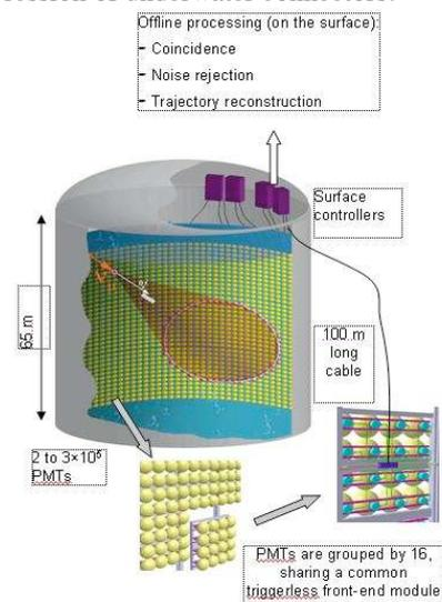
Fig .1. Principal of PMm<sup>2</sup> proposal for megaton scale Cerenkov water tank with 16 PMTs array shown in the bottom side of the picture and are emphasized the surface controller and the 100m of cable.
