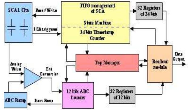
Fig. 5. Block diagram of the digital part.
