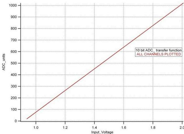
Fig. 19. 10-bit ADC transfer function vs input charge.
