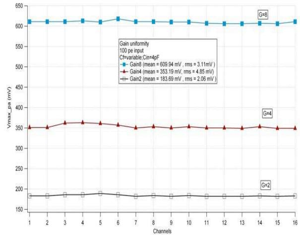
Fig. 11. Gain uniformity for  $G_{pa} = 8, 4, 2$ .
