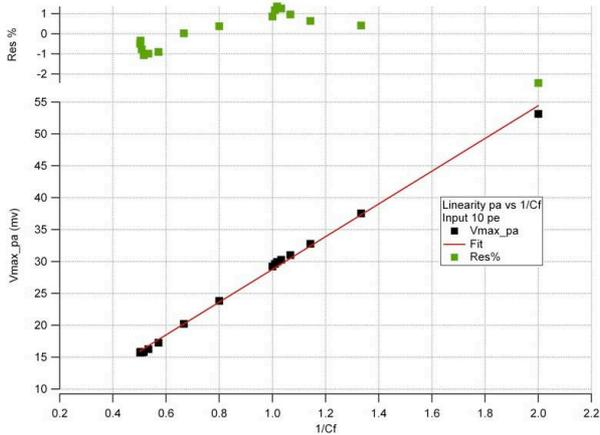
Fig. 9. Preamplifier linearity vs feedback capacitor value.
