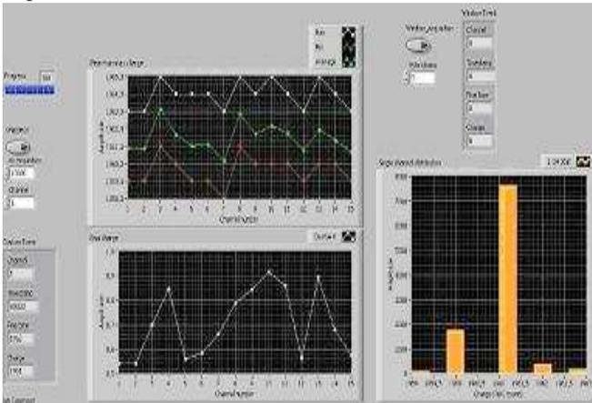
Fig. 18. ADC measurements with DC input 1.45V.
