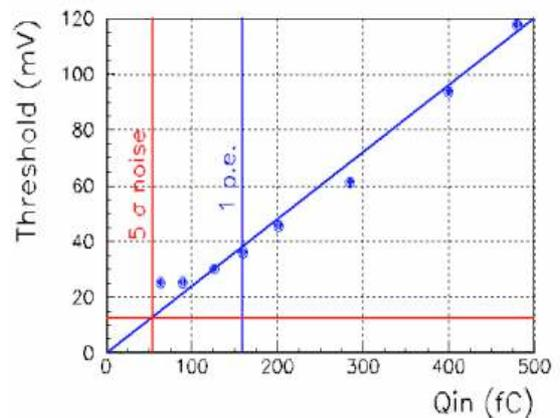
Fig. 17. Threshold vs injected charge until 500 fC.
