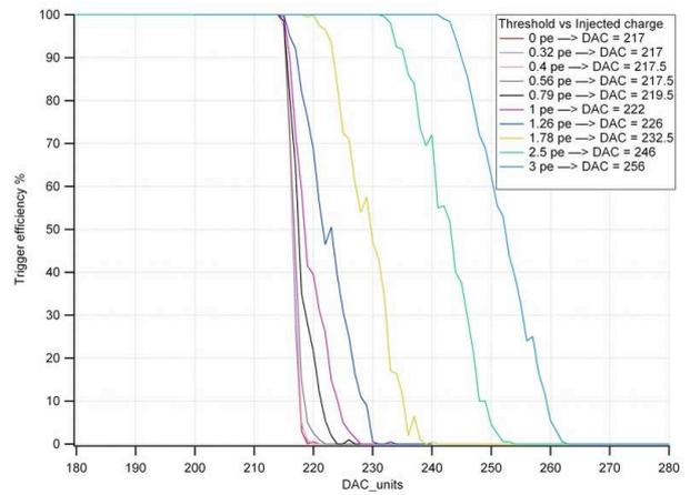
Fig. 16. Trigger efficiency vs DAC count until 3 p.e.
