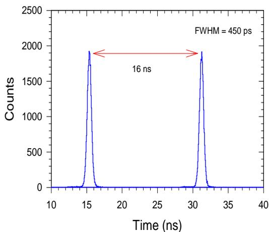
Fig. 6. Time resolution of individual detector using  $^{60}\text{Co}$   $\gamma$ -source.
