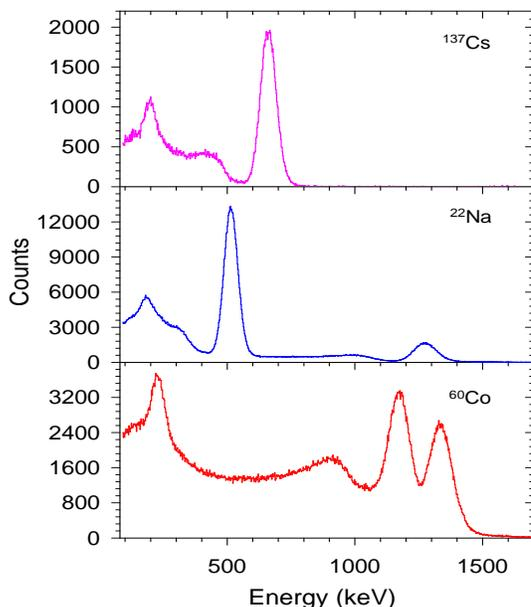
Fig. 5. Energy spectra from a single detector for different lab. standard gamma ray sources.
