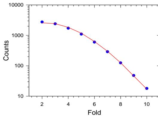
Fig. 11. Experimental fold spectrum (symbols) fitted with GEANT simulation (solid line) for  $^{252}\text{Cf}$  source.
