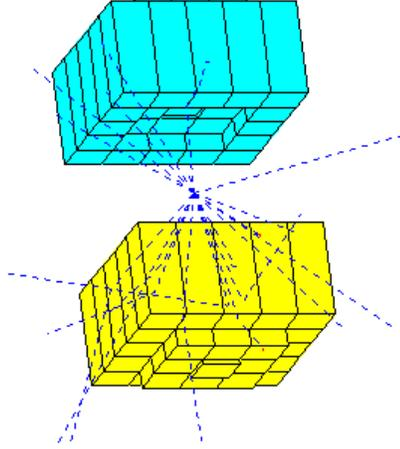
Fig. 1. Schematic view of the multiplicity filter array GAMMA in castle type geometry.
