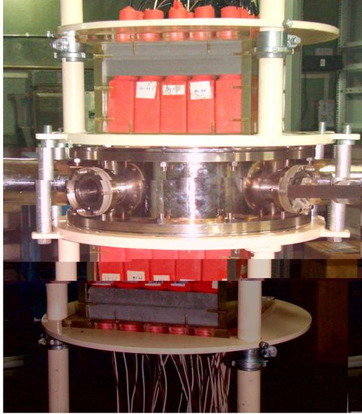
Fig. 4. Complete setup of the multiplicity filter array GAMMA kept on either side of the scattering chamber.
