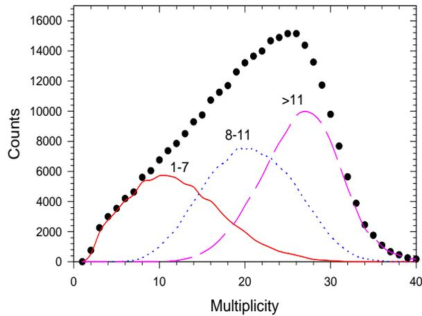
Fig. 8. The sampling of the total angular momentum distribution by gating on different folds observed in the fold distribution of the multiplicity filter.
