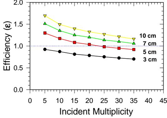
Fig. 2. Multiplicity detection efficiency vs. incident multiplicity plot for various detector lengths.
