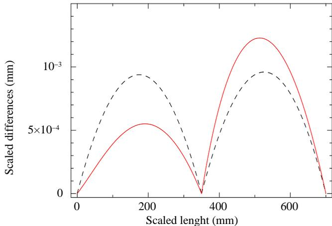
**Figure 3.** Differences between a Wolter I (dashed) or a polynomial (continuous) mirror shell with respect to a double cone profile for a  $f = 5$  and  $l = 7$  mirror and with focal length  $F = 1000$  mm.
