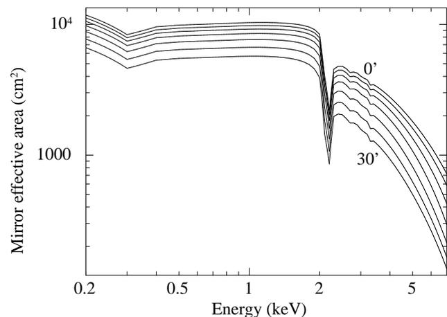
**Figure 11.** Effective area for the full telescope (three mirror units) discussed in the text, including 10% obstruction from the support structure. From top to bottom areas are for  $0'$  to  $30'$  off-axis angles in step of  $5'$ .
