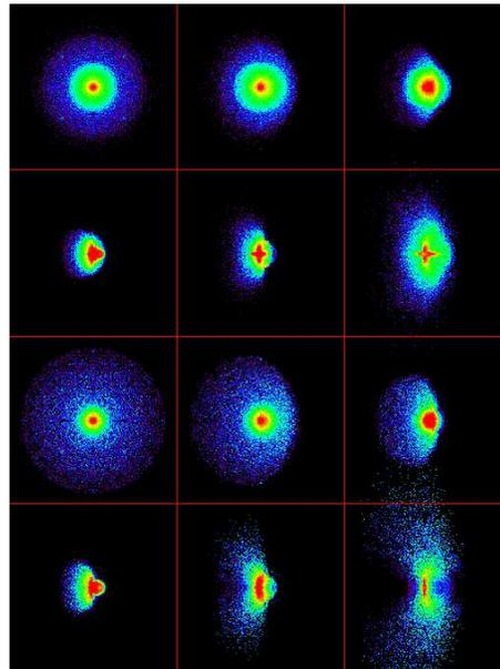
**Figure 10.** Full telescope spot at 1 keV (6 upper panels) and 4 keV (6 lower panels) at off-axis angles of  $0'$ ,  $6'$ ,  $12'$ ,  $18'$ ,  $24'$  and  $30'$ , respectively, evaluated on the best (inverse pyramid) CCD focal plane. Surface roughness has not been considered. Images are 20 arcsec apart.
