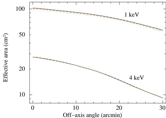
**Figure 9.** Effective areas of the unitary telescope (focal length  $F = 1000$  mm) for the three designs discussed in the text at two different energies over the field of view at 1 keV and 4 keV. Continuous lines refer to  $l = 8$  (initial value for the outermost shell), dashed lines to  $l = 7$  and dotted lines to  $l = 6$ .
