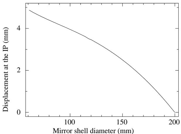
**Figure B2.** Displacements at the intersection plane (IP) in mm to align each mirror shell spot on the inverse pyramid focal plane as a function of the mirror entrance diameter. Numbers refer to the unitary telescope with  $F = 1000$  mm.
