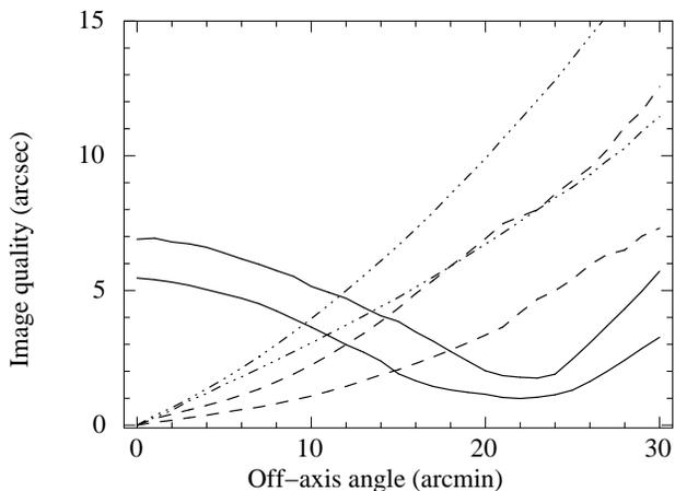
**Figure 4.** Image quality functions over the field of view for different mirror shells with  $f=5$  and  $l = 7$ . Dot-dot-dot-dashed lines refer to the Wolter I, dashed lines to Wolter-Schwarzschild and continuous lines to the polynomial mirror. The two different lines for each mirror type are (from bottom to top), HEW and 80% EEf.
