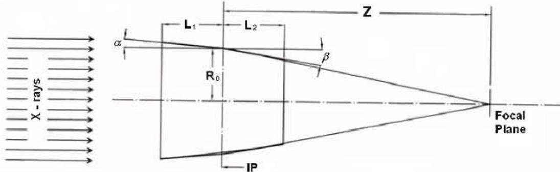
**Figure 1.** Telescope configuration and parameters.  $R_0$  is the mirror shell radius at the intersection plane (IP);  $\alpha$  ( $\beta$ ) is the angle the between the primary (secondary) mirror tangent at the intersection plane and the optical axis;  $L_1$  ( $L_2$ ) is the length of the parabola (hyperbola) mirror segment;  $Z$  is the distance between the IP and the focal plane along the optical axis. For an X-ray telescope  $Z$  is very close to the focal length of the telescope  $F$ .
