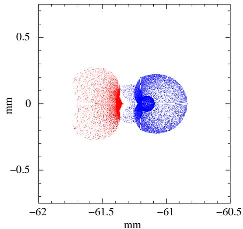
**Figure B1.** Image spot of two different shells (outermost and innermost) at an off-axis position of 20' at 1 keV taking the same focal length for the two shells. This blur is corrected changing the focal length of the innermost shell and then shifting it at the intersection plane to achieve the same plate scale as the outermost. the shift at the intersection plane. In this configuration 1 mm in the focal plane corresponds to 20 arcsec.
