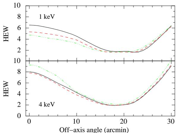
**Figure 8.** HEW for the three designs discussed as a function of the off-axis angle. In the top panel are shown the HEW at 1 keV: the continuous line refers to the  $l = 8$  (initial value for the outermost shell) design, the dashed line to  $l = 7$ , and dash-dot-dotted line to  $l = 6$ . In the lower panel the same curves are shown for an energy of 4 keV. All the curves were obtained without considering scattering due to microroughness.
