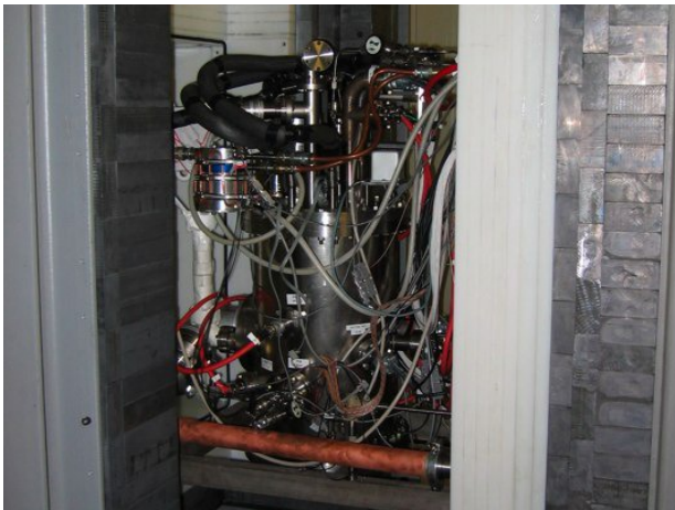
FIG. 4: (Color online) Photo of the XENON10 detector and shield, with the shield door open.
