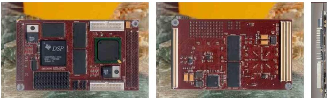
Figure 3.3: Photos of the SMT361 DSP/FPGA Processor Module
