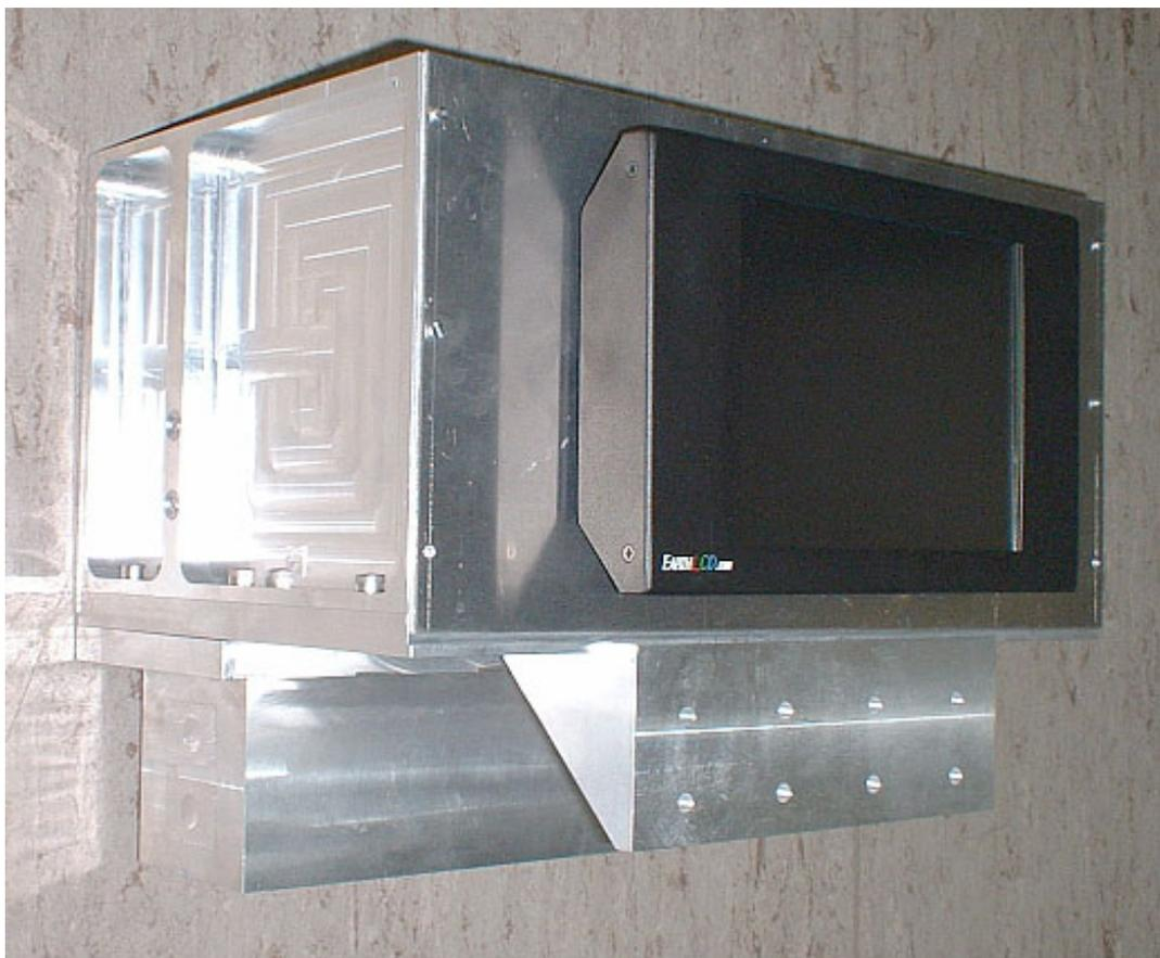
Figure 5.4: Side view of the aluminum detector housing with integrated industrial LCD monitor
