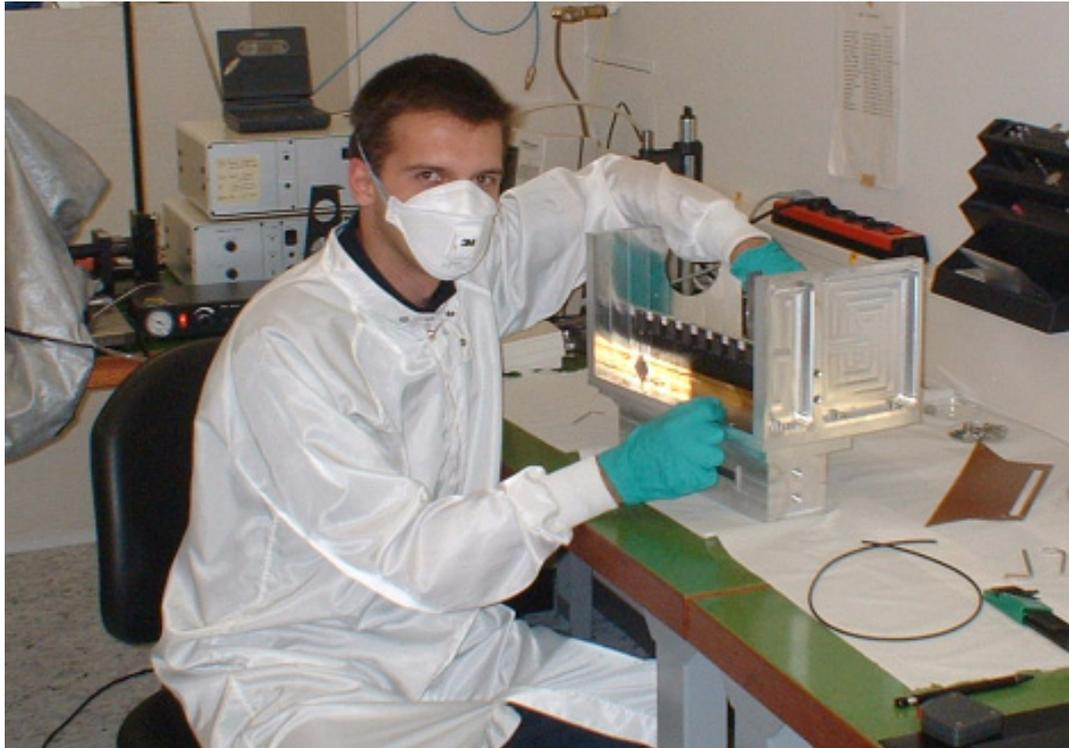
Figure 5.5: Picture showing a preliminary mounting of the SAXS Hybrids on the anode, performed in the *clean room* of the FEC Group at DESY, Hamburg
