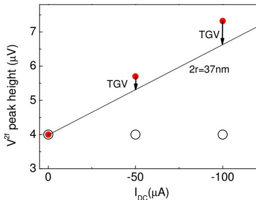
FIG. 4:  $V^{2f}$  peak height as a function of  $I_{dc}$ , for fixed  $I_{ac}=100 \mu\text{A}$ . The dots (red) are the experimental data for an asymmetric spin valve. The open circles (black) are the experimental data for a symmetric spin valve. The arrows indicate a linear correction to the data of the asymmetric spin valve by subtraction of an estimated value for the TGV. The line (black) is a calculation using the nanowire diameter of 37 nm as indicated in the text.
