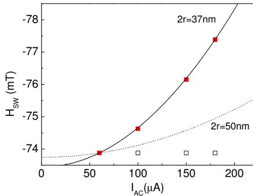
FIG. 3: Switching field measured as a function of  $I_{ac}$ , for fixed  $I_{dc} = -100 \mu\text{A}$ . Squares (red) are the experimental data for an asymmetric spin valve. The open boxes (black) are the data for a symmetric spin valve. The lines (black) are the result of calculations with different nanowire diameters as indicated in the text.
