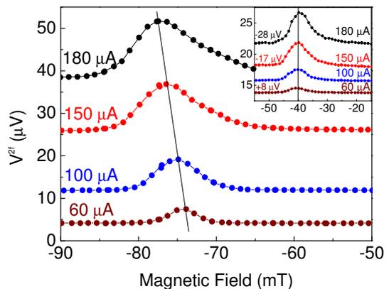
FIG. 2:  $V^{2f}$  measurements on a nanowire containing an asymmetric spin valve (10 nm Co/10 nm Cu/30 nm Co) at a set dc current of  $-100 \mu\text{A}$  for different values of the ac current, as indicated in  $\mu\text{A}$ . The field was swept from negative to positive values. Inset: idem for a symmetric spin valve (10 nm Co/10 nm Cu/10 nm Co). Curves are offset vertically by the values specified in  $\mu\text{V}$ . The lines are guides for the eye.
