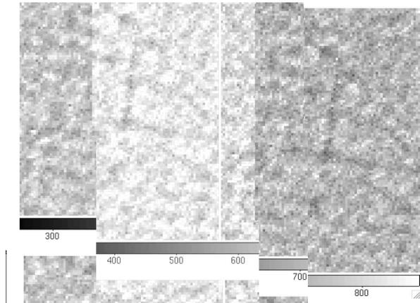
**Figure 11.** Persistent small scale structure shows up in the UVOT flat fields, made using the onboard LED lamp. The SSS refers to the dark lines and patches over and above the regular mod8 noise. This is a comparison between data taken in 2005 (left) and 2008 (right). Each of these images is  $120 \times 90$  pixels.
