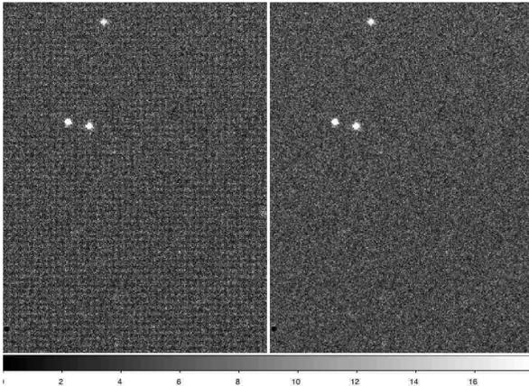
**Figure 8.** Part of a raw *white* image before (left) and after (right) correction by UVOTMODMAP. The mod-8 patterning shows up as a faint grid in the left hand image. Each of these images is  $470 \times 340$  pixels.
