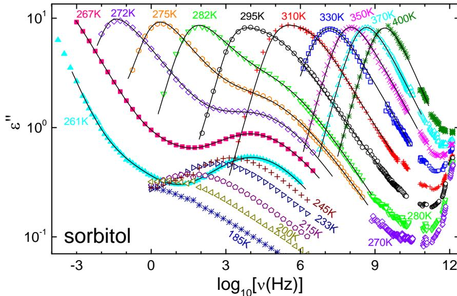
Fig. 2. Broadband dielectric loss spectra of glass forming sorbitol at selected temperatures. The lines are fits with the sum of a Havriliak-Negami and a Cole-Cole function.
