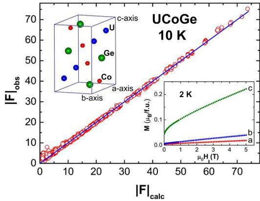
FIG. 1: (Color online) Observed *versus* calculated nuclear structure factors after correction for absorption and extinctions of the UCoGe single crystal in the unpolarized neutron diffraction experiment at  $T = 10$  K. Upper inset: Schematic representation of the TiNiSi structure adopted by UCoGe. Lower inset: Magnetization *versus* magnetic field of UCoGe at  $T = 2$  K for a magnetic field applied along the three principal axes<sup>8</sup>.
