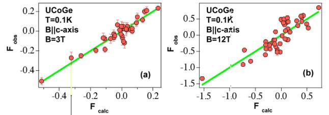
FIG. 2: (Color online) Observed *versus* calculated (solid line) magnetic structure factor of UCoGe for the polarized neutron diffraction experiment at  $T = 0.1$  K in an applied field ( $B \parallel c$ ) of 3 T (a) and 12 T (b).
