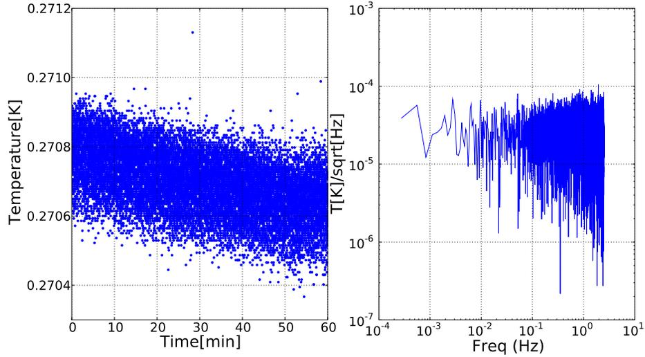
Fig. 5. Left: A measurement of the temperature of the 410 GHz wafer during an azimuth scan with a peak to peak amplitude of up to  $120^\circ$  at a scan speed of  $0.5^\circ/\text{s}$ . Right: Power spectrum of the temperature data after removing an offset and gradient.
