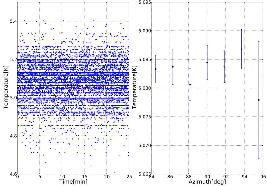
Fig. 4. Left: A measurement of the temperature of the liquid helium tank during a sinusoidal azimuth scan with a peak-to-peak amplitude of  $9^\circ$  and a period of 25 s. Right: The time ordered data from the left panel binned and plotted vs. azimuth.
