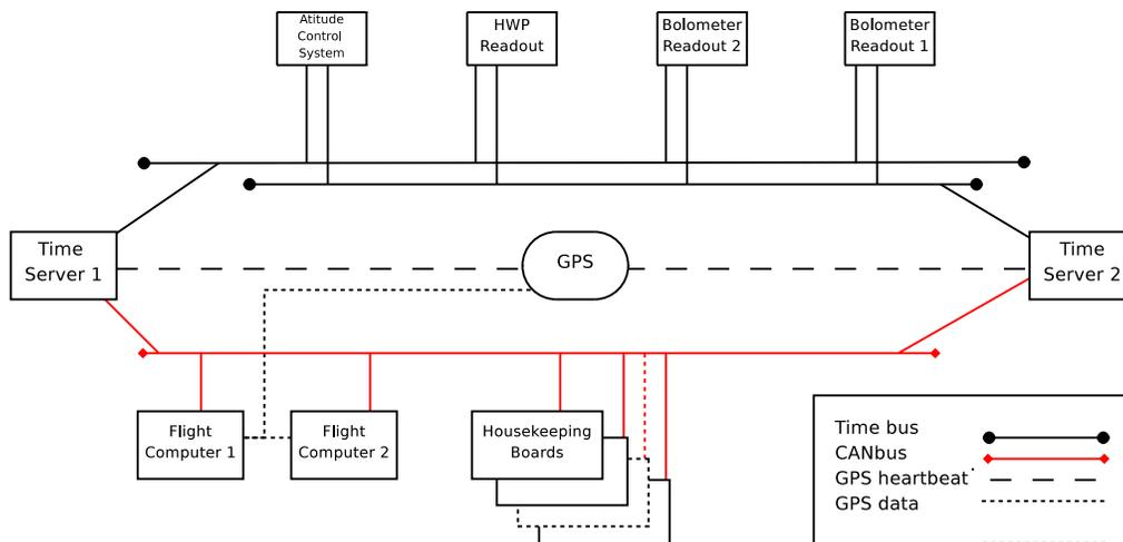
Fig. 6. The EBEX time bus. The black line represents the RS-485 time buses.
