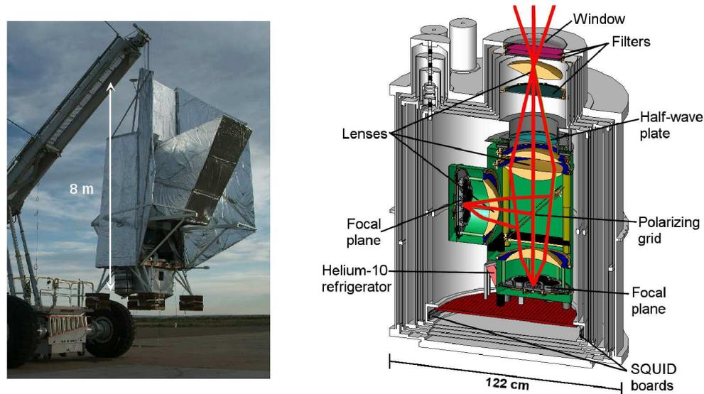
Fig. 1. Left: The EBEX payload before launch. Right: A cross section of the EBEX cryostat.
