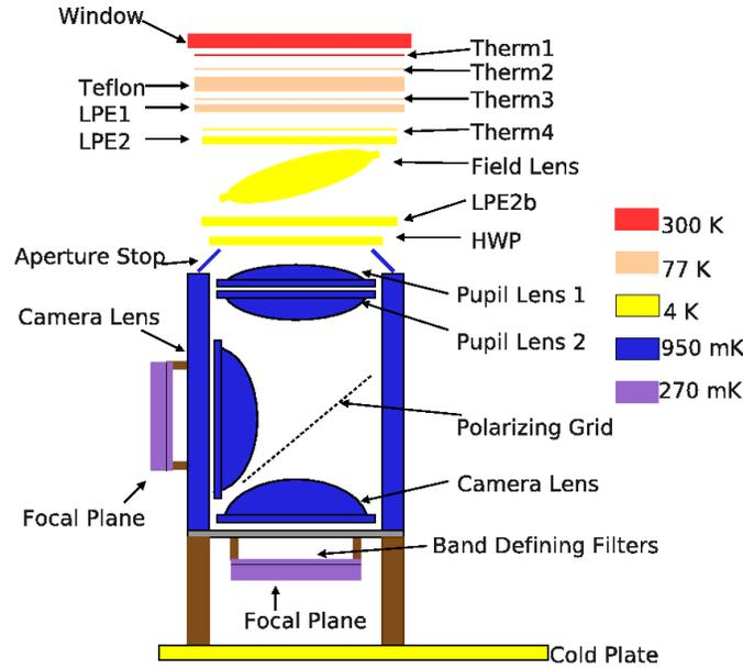
Fig. 2. EBEX cold optics color coded by temperature
