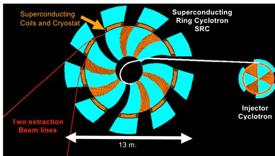
Figure 3.2: Schematic of the Multi-MegaWatt Cyclotron
