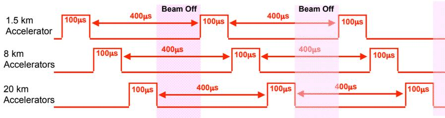
Figure 2.2: The source accelerator for events is identified through timing. We propose to run each accelerator with a 20% DF. Beam-off time allows measurement of non-beam-backgrounds. The timing structure presented here is illustrative, and longer intervals are not an issue for the analysis.
