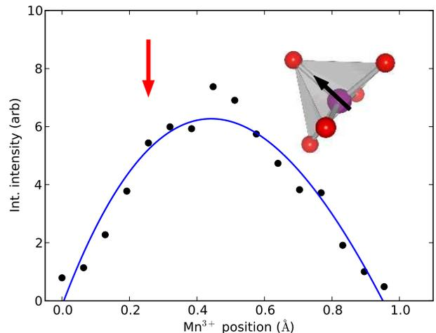
FIG. 4. The integrated intensity of the calculated resonance through varying the  $\text{Mn}^{3+}$  position toward the apical oxygen, out of the basal plane (schematic). The solid line is a guide to the eye, and the vertical red arrow indicates the empirically determined position of the  $\text{Mn}^{3+}$  ion[9].
