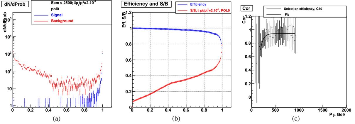
Figure 4: (a) (left panel) distribution of the combined probability variable for signal events (blue) and background events (red);  $\delta p_t/p_t^2 = 2 \times 10^{-5} \text{ GeV}^{-1}$ , (b) (middle panel) efficiency and S/B as a function of the probability value without polarisation, (c) (right panel) selection efficiency for a probability cut larger than 0.8 as a function of muon momentum.
