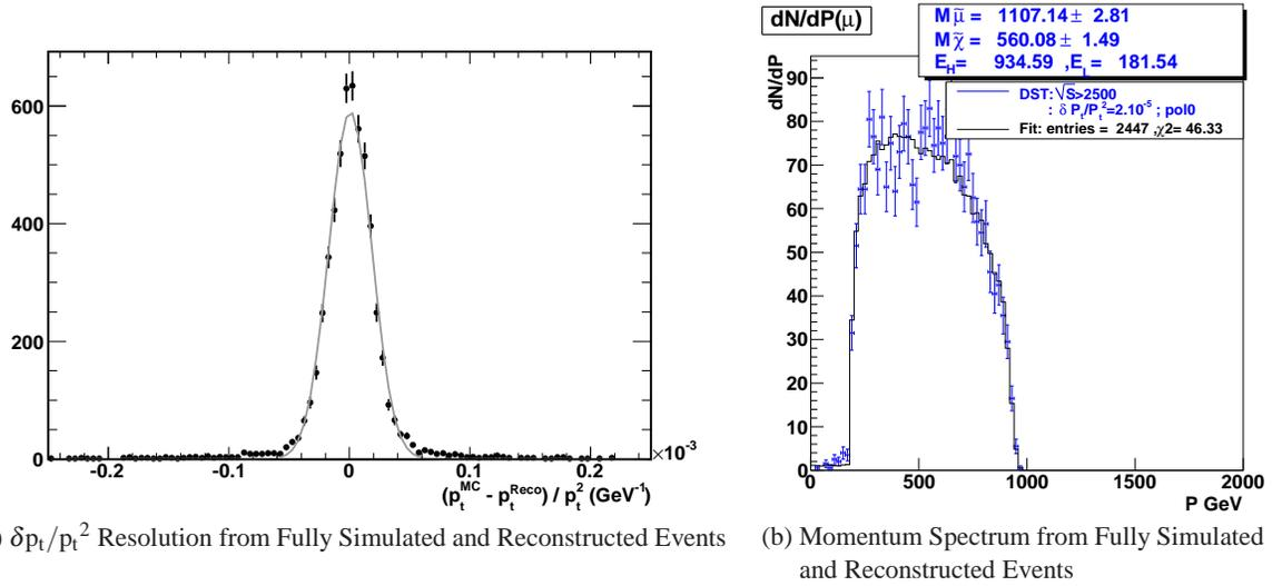
Figure 14: Validation using fully simulated and reconstructed events for the CLIC01-ILD detector. (Left) Distribution of the difference between the generated and reconstructed  $p_t$  of muons normalised to the squared  $p_t$  ( $\delta p_t/p_t^2$ ), after full simulation and reconstruction. The width of the fitted Gaussian curve is  $1.8 \times 10^{-5} \text{ GeV}^{-1}$ . (Right) Fit to the signal muon momentum spectrum.
