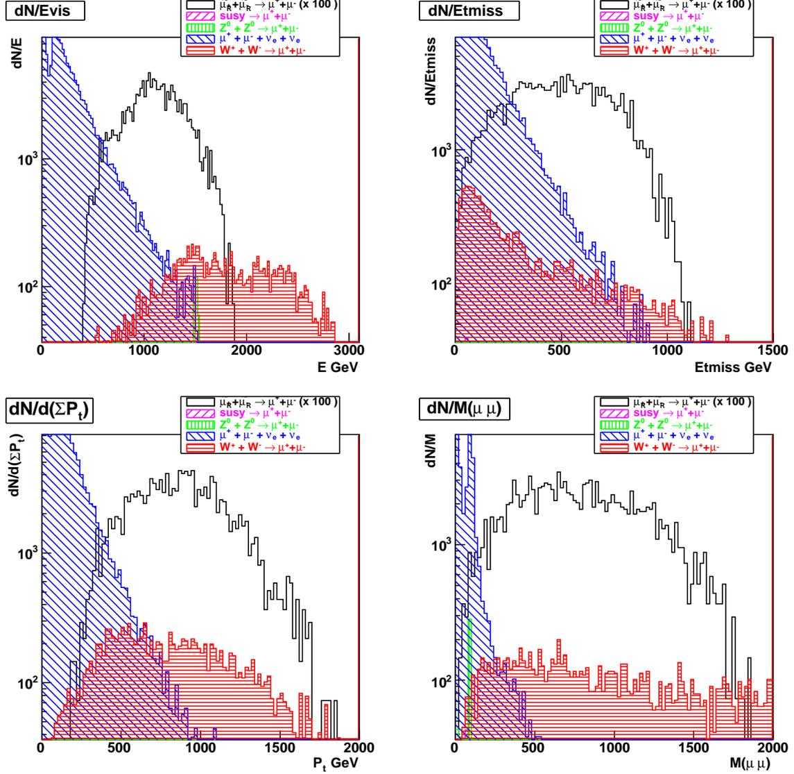
Figure 2: Discriminating variables used in the combined likelihood function: (upper left)  $E_{\text{vis}}$  visible energy, (upper right)  $E_{\text{miss}}$  missing transverse energy, (lower left)  $\sum p_t$  sum of the  $p_t$  of the muons and (lower right)  $M_{(\mu\mu)}$  invariant mass of the two muons
