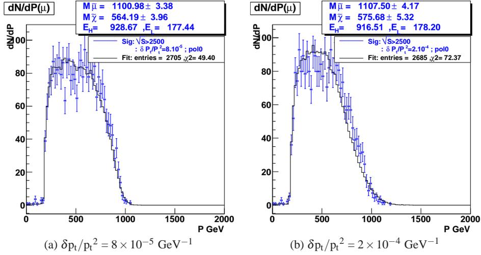
Figure 11: Fits to the signal muon momentum spectrum for momentum smearing of (a)  $\delta p_t/p_t^2 = 8 \times 10^{-5} \text{ GeV}^{-1}$  and (b)  $\delta p_r/p_r^2 = 2 \times 10^{-4} \text{ GeV}^{-1}$ .
