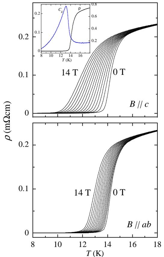
FIG. 6. (color online) Resistivity versus temperature for sample 1 for fields between 0 and 14 T applied either parallel or perpendicular to  $c$ . The inset in the upper panel shows a direct comparison of the resistivity (left hand scale) and heat capacity (right hand scale) of the same sample (sample 1) in zero magnetic field.
