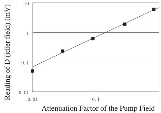
Fig. 2. The detected signal size of the “idler” field as a function of the attenuation factor of the pump field or the transmission coefficient of the attenuator ATT. The solid line is  $y = ax$  with  $a = 7$  for best fit.
