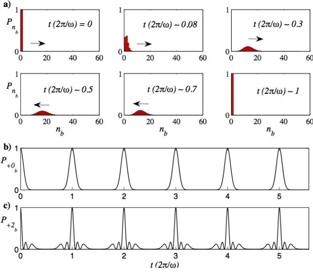
FIG. 1. (Color online) (a)-(b) Round trip of a photon number wavepacket and collapse-revivals due to DSC dynamics with initial state  $|+, 0_b\rangle = |g, 0_a\rangle$ . c) Collapse-revivals with secondary peaks due to counterpropagating photon number wavepackets starting in initial state  $|+, 2_b\rangle = |g, 2_a\rangle$ . For all cases,  $\omega_0 = 0$  and  $g/\omega = 2$ .
