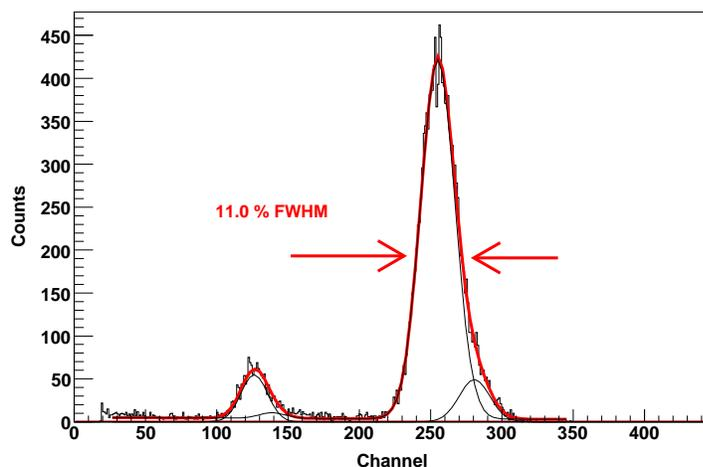
**Figure 1.** Typical spectrum of  $^{55}\text{Fe}$  with a microbulk Micromegas in an argon-isobutane mixture. The red line is the result of a fit to 4 Gaussians, while the thin black lines are the 4 Gaussians separately, corresponding to the two x-ray emission lines of  $^{55}\text{Fe}$  of 5.9 and 6.5 keV, and their corresponding escape peaks in argon.
