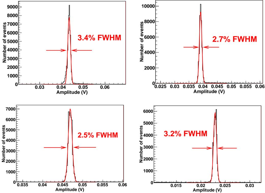
**Figure 6.** Energy spectra of the  $^{241}\text{Am}$  alpha peak measured in the setup at 2 (top left), 3 (top right), 4 (bottom left) and 5 bar (bottom right). The red line and the value for the energy resolution are the result of the fit to a Gaussian function.
