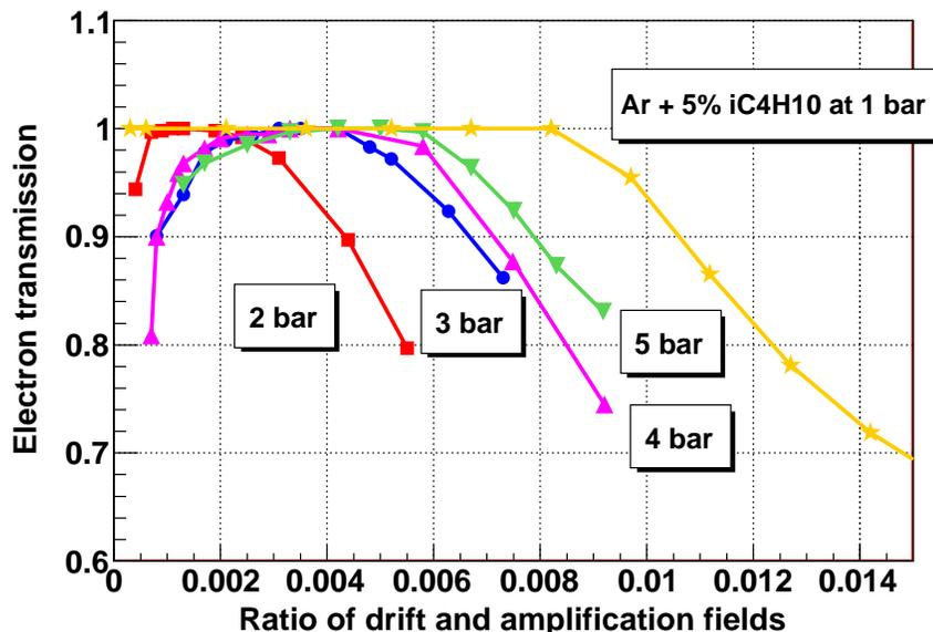
**Figure 5.** Dependence of the alpha peak position on the ratio of drift and amplification fields (*electron transmission curve*) at 2 (red squares), 3 (blue circles), 4 (magenta triangles) and 5 bar (inverted green triangles). As a comparison, the same curve for Ar + 5% iC<sub>4</sub>H<sub>10</sub> at 1 bar (yellow stars) is included. Values are normalized to the maximum of each series.
