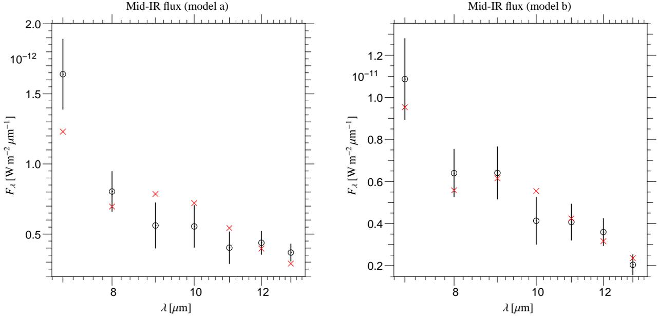
**Fig. 3.** Simulated VLTI/MIDI mid-IR object flux. The numerically generated data (left model a, right model b) are shown as circles with error bars. The values of the fluxes for the best-fit models are represented as crosses.
