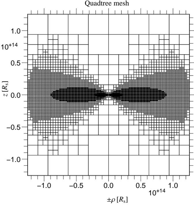
**Fig. 2.** Quadtree mesh for a disc configuration. The disc parameters are those of model (b) described in Sect. 5.2 (see also Tables 2 and 4). The mesh refinement parameter  $\eta$  (Eqs. 7 and 8) has been set to the high value  $10^{-3}$  in order to obtain a coarse mesh more easily represented.
