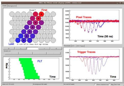
Figure 3: Monte Carlo simulated detection of an EAS with the MIDAS experiment. Shower energy is  $1.15 \times 10^{19}$  eV shower maximum located 15.2km from the detector. Left panels show time structure and geometry for the event. The upper right panel displays the raw traces from selected channels and lower right panel displays the  $1\mu\text{s}$  running sum trace which the system uses for triggering.
