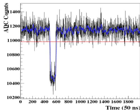
Figure 2: Single channel output of a pulse from log-period antenna used for calibration. Signal is inverted due to reverse voltage bias of power detector. Black trace is raw output from channel. Blue trace is the  $1\mu\text{s}$  running sum. Red Line represents the threshold level.
