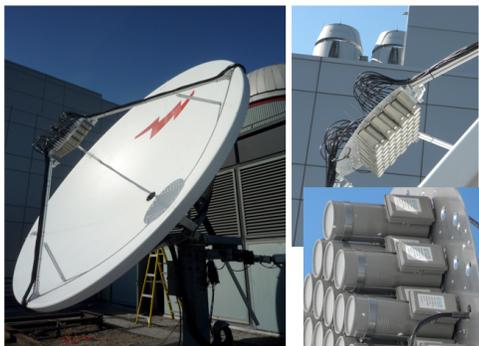
Figure 1: Left: 4.5 m parabolic reflector with 53 channel camera mounted at the the prime focus. Right: Close-up view of 53 channel camera in reflector's focal plane.
