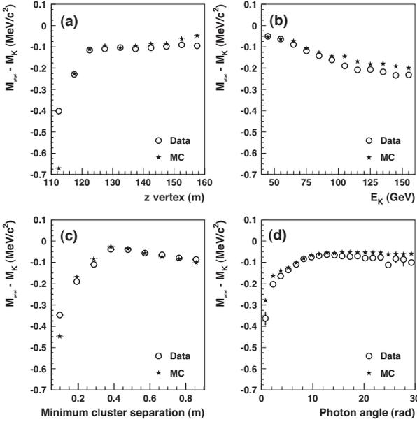
FIG. 17: Comparisons of the reconstructed kaon mass vs (a)  $z$ -vertex, (b) kaon energy, (c) minimum cluster separation, and (d) photon angle for 1999 data (circles) and MC (stars). The values plotted are the difference between the reconstructed kaon mass for each bin and the PDG kaon mass.
