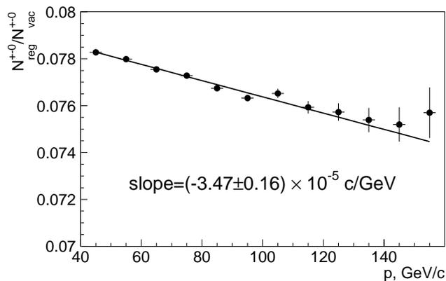
FIG. 20: Ratio of  $K_L \rightarrow \pi^+\pi^-\pi^0$  decay rates in the regenerator to vacuum beam as a function of a kaon momentum. The uncertainty on the slope is statistical uncertainty of the measurement.
