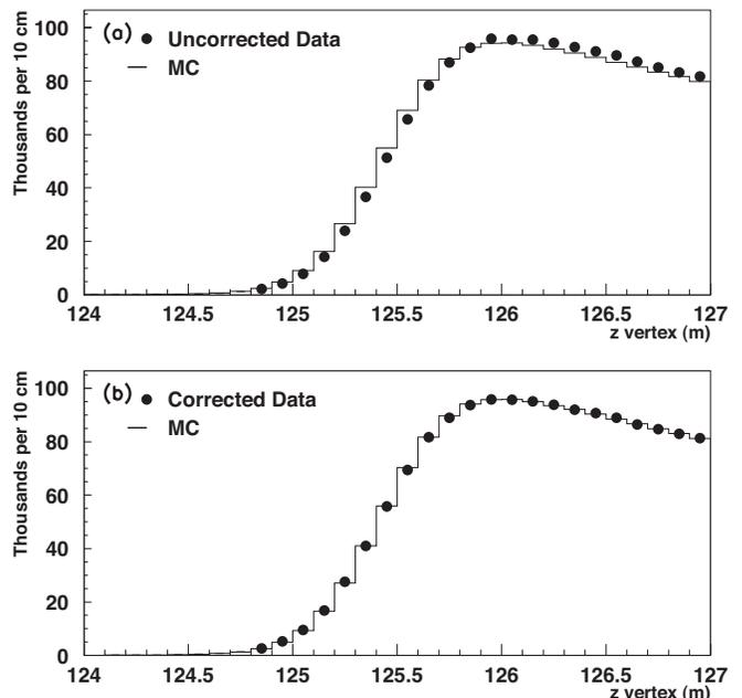
FIG. 13: Regenerator beam  $K \rightarrow \pi^0 \pi^0$   $z$  vertex distribution near the regenerator for 1999 data and Monte Carlo. (a) Uncorrected data. (b) Data with energy scale correction applied.
