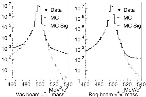
FIG. 8:  $\pi^+\pi^-$  invariant mass distribution for  $K \rightarrow \pi^+\pi^-$  candidate events in the vacuum (left) and regenerator (right) beams. The data distribution is shown as dots, the  $K \rightarrow \pi^+\pi^-(\gamma)$  signal MC (MC Sig) is shown as dotted histogram and the sum of signal and background MC is shown as a solid histogram.
