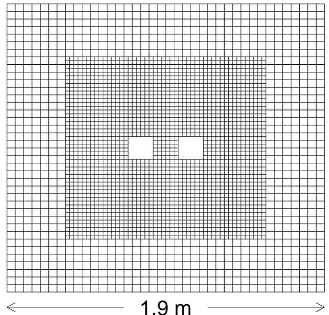
FIG. 5: Beamline view of the KTeV CsI calorimeter, showing the 868 larger outer crystals and the 2232 smaller inner crystals. Each beam hole size is 15  $\times$  15 cm<sup>2</sup> and the two beam hole centers are separated by 0.3 m. The positive  $z$  direction is into the page.
