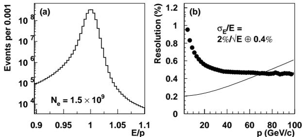
FIG. 10:  $K_{e3}$  electrons after all corrections. (a)  $E/p$  for  $1.5 \times 10^9$  electrons. (b) Energy resolution. The fine curve shows the momentum resolution function that has been subtracted from the  $E/p$  resolution to find the energy resolution.
