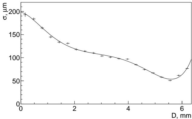
FIG. 7: Dependence of drift chamber position resolution on position within the cell.  $D$  is the distance from the sense wire. Crosses represent the measured central values and uncertainties of the resolution in bins of  $D$  and the line represents a polynomial fit to the data. This fit is used in the simulation to parameterize the position dependence of the position resolution.
