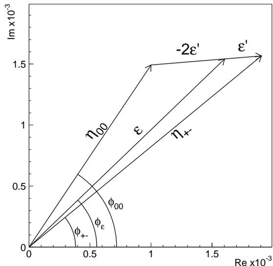
FIG. 1: Diagram of CP violating kaon parameters. For this illustration, the  $\epsilon$  parameter has the central value measured by KTeV and the value of  $\epsilon'$  is scaled by a factor of 50. Although they appear distinct in this diagram, note that  $\phi_{+-}$  and  $\phi_{00}$  are consistent with each other within experimental errors.
