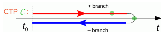
Fig. 1. Schwinger-Keldysh closed time path \mathcal{C} . The green dots indicate the times x_0 and y_0 for an example two-point function \langle \Phi(x)\Phi(y) \rangle , see text. The branches are drawn above and below the time axis to make them separately visible.
