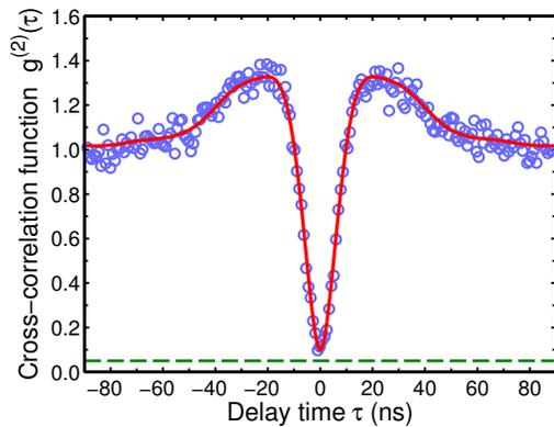
FIG. 4. (color online). Normalized cross-correlation signal  $g^{(2)}(\tau)$  of photon arrival times at the end of the two fibers. The dashed line indicates the expected background level due to stray light and dark counts, which have not been subtracted. The excellent agreement with the superimposed numerical solution of the master equation demonstrates the distinct quantum character of the emitted radiation.
