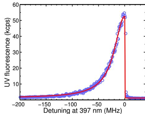
FIG. 3. (color online). Fluorescence spectrum of a single ion in the fiber-coupled endcap trap. Excitation and repumping beams at a power of 0.39  $\mu\text{W}$  (equivalent to an intensity of  $1.3I_s$ ) and 0.5 mW, respectively, are injected from the side of the trap. The combined fluorescence of the two fibers is plotted and no background subtracted. It is fit by a Lorentzian with a half width of 23.8 MHz (solid line).
