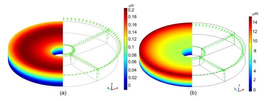
Figure 7: A snapshot of the surface distortion of (a) Zerodur mirror (b) SiC mirror for  $(0-10^{\circ}\text{C})$  ambient temperature change. The direction of the displacement vectors at the mirror surface is denoted by arrows shown in green.
