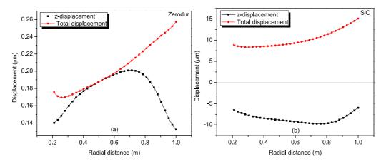
Figure 8: Calculated displacement along the top surface of (a) Zerodur (b) SiC mirror.
