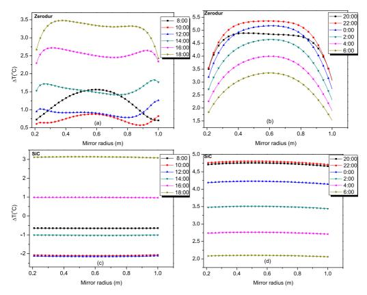
Figure 5: Radial temperature difference of the front mirror surface during day-time and night-time for (a)–(b) Zerodur mirror and (c)–(d) for SiC mirror. The ambient temperature range is  $0 - 10^{\circ}$ C.
