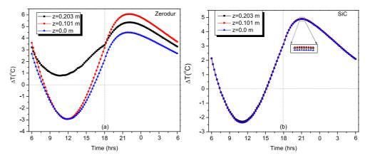
Figure 4: Differential temperature variations evaluated for a reference point on top, middle and bottom of (a) Zerodur (b) SiC mirror. The ambient temperature range is  $0-10^{\circ}$ C.
