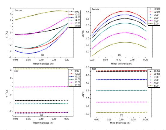
Figure 6: Axial temperature difference along the thickness of the mirror blank during day and night-time for (a)–(b) Zerodur material, and (c)–(d) for SiC. The ambient temperature range is  $0-10^{\circ}$ C.
