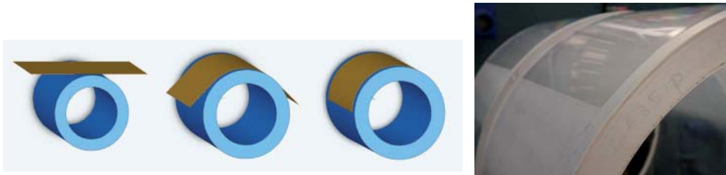
Figure 4.5. Left: Graphic illustration of the glass slumping process. Right: this panel shows two mandrels with substrates on them that have come out of the oven.
