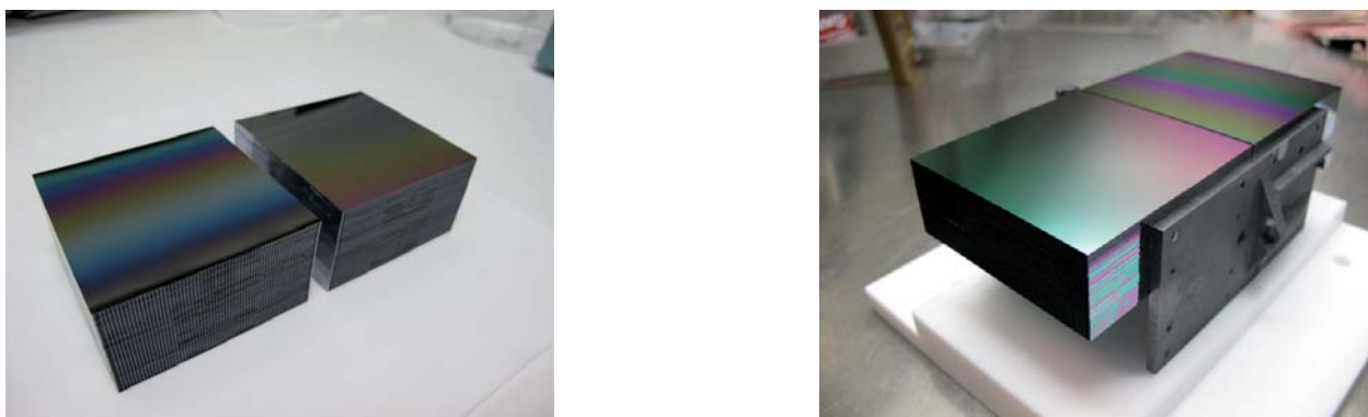
Figure 4.3. Left: a pair of SPO stacks, consisting of 45 bonded mirror plates each, as required for the IXO telescope baseline design. Right: A complete SPO mirror module, consisting of a pair of mirror plate stacks permanently joined by two CTE matched silicon carbide brackets (cosine Research BV).
