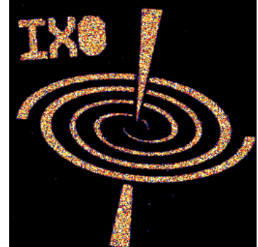
Figure 4.18. X-ray image taken by the DEPFET matrix shown in Figure 4.17, demonstrating the high resolution of this prototype.
