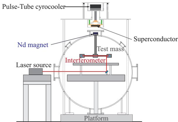
FIG. 2: Conceptual design of small-scaled TOBA.
