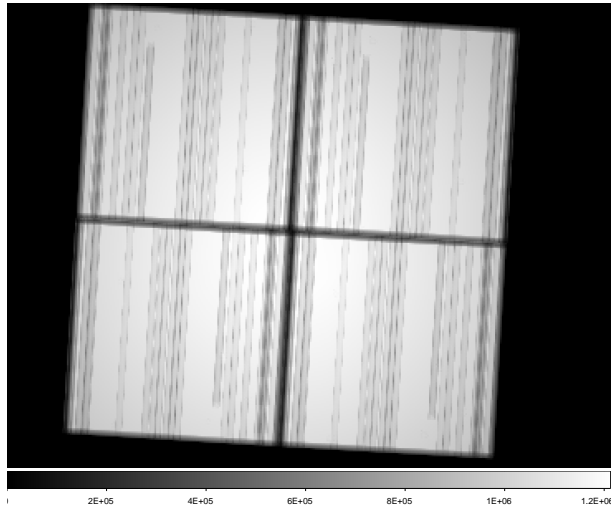
FIG. 5.— The exposure map for the observation with Obs ID 9999 for an assumed mono-chromatic source emitting 1 keV photons, showing the lower exposure for the gaps between the ACIS I CCDs. Lighter areas have a higher exposure on the sky (in terms of \text{cm}^2 \text{ s}^{-1} ). Due to the satellite dithering some exposure is achieved even for the gaps. The vertical strips are caused by the presence of columns of pixels of reduced efficiency. The grey area is approximately 8' \times 8' in size.
