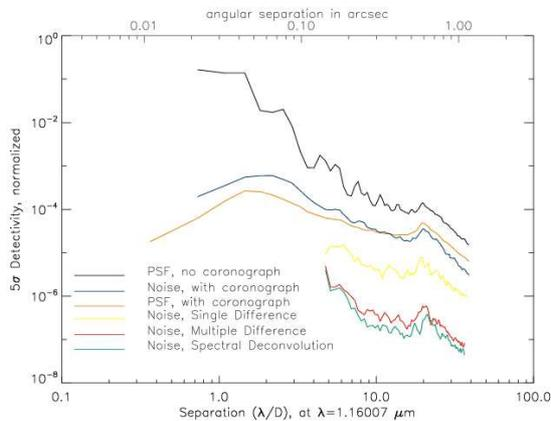
**Fig. 6.** Run of the  $5\sigma$  calibration limit with separation for a very bright star. The case shown is for  $30^\circ$  field rotation with azimuthal filtering. Detector noises and a cross-talk with a value of  $10^{-2}$  were introduced too. Red line is the result obtained with multiple differential imaging while the green is with the spectrum deconvolution method.
