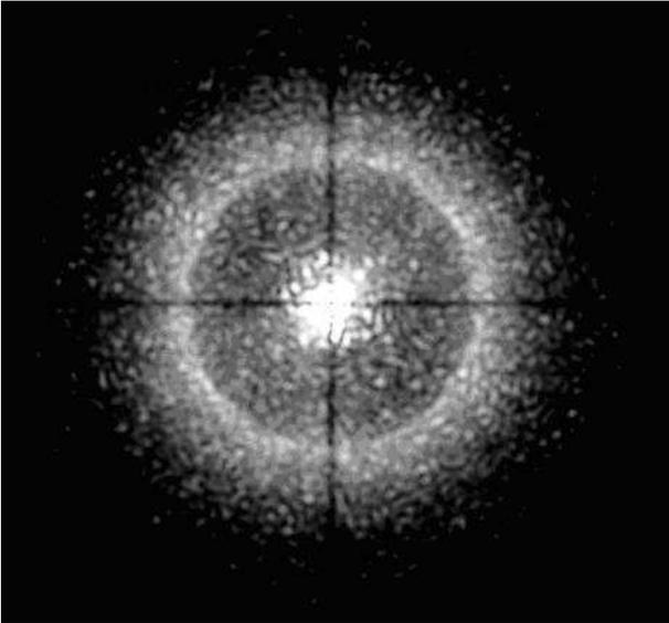
**Fig. 1.** Monochromatic PSF resulting from the CAOS simulation. The bright corona corresponds to the outer working angle of the XAO system. Its radius is roughly 0.5 arcsec at the working wavelength. This image has been obtained using a 4-quadrant coronagraph. The cross structure centered on the center of the image is the signature of this type of coronagraph.
