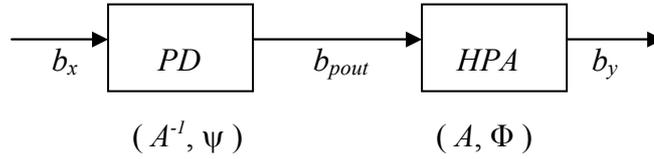
Fig. 3. Pre-distortion For HPA Linearization
