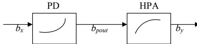
Fig. 4. Basic System Functional Diagram of Pre-distortion Linearization
