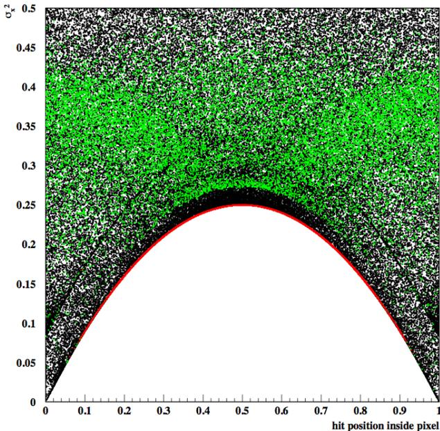
FIG. 7: Results of  $\hat{x}$  and  $\hat{\sigma}_x^2$  for 5.9 keV X-rays on front (red) and back (green) of a CCD. The black data corresponds to hits from the same  $^{252}\text{Cf}$  source shown in Fig.4. As expected from simulations the back illuminated X-rays produce hits with large  $\hat{\sigma}_x^2$ , while the front illuminated X-rays are very close to the boundary defined by Eq.1.
