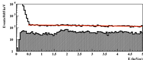
FIG. 8: Measured spectrum for  $^{252}\text{Cf}$ . The upper line shown the raw data without applying any selection criteria, the lower hatched histogram shows the result after selecting hits with intermediate size. The raw data is fitted to a linear function above 0.5 keV.
