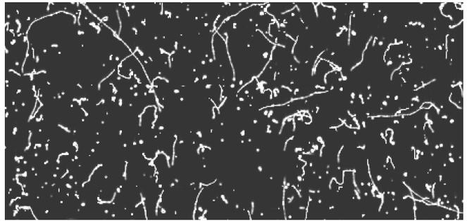
FIG. 4: Image resulting from an exposure of a DECam CCD to a  $^{252}\text{Cf}$  neutron source. The total width of the image corresponds to 1000 pixels. The smaller dots represent the diffusion-limited hits, the trails correspond to scattered electrons and there is one bigger circular cluster of charge that corresponds to an alpha particle.
