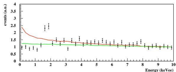
FIG. 5: Reconstructed electron equivalent energy spectrum for  $^{252}\text{Cf}$  exposures. The data is consistent with expectations from Lindhard theory (red). The expectations for an energy independent quenching factor are also shown for comparison (green).
