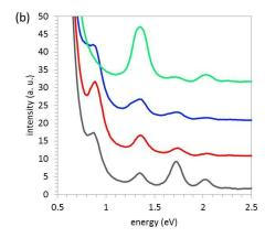
Figure 1. (a) Bright-field (BF) zero-loss image of a 666±3 nm long silver nanorod, with 47±3 nm diameter. (b) Electron energy-loss spectra (unprocessed) acquired at the positions marked in (a) of matching colour. Spectra have been obtained using a selected-area approach [18] and shown displaced on the intensity axis for clarity.
