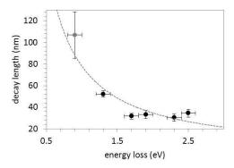
Figure 4. Decay length *D* as a function of energy loss for the SP resonant modes probed experimentally in Figure 2. Horizontal error bars are defined by the 0.23 eV energy filter window. The dashed grey line fits a power law function with exponent -1.
