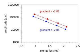
Figure 5. Plot of the intensity (area of the fitted Gaussian of the individual SP peaks in the spectrum of Figure 1(b) in blue and red) at the right tip (red circles) and left tip (blue circles) of the nanorod as a function of energy loss. It is clear that the intensity follows an exponential decay, with exponent of approximately -2. The error in the measurement of intensity is not shown as it is smaller than the size of the markers.
