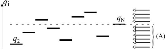
FIG. 3. An example of the distribution, where there are five upward steps ( $n = 6$ ) and five offset charges less than  $q_N$  ( $k = 5$ ). The arrows at right indicate the possible location of  $q_{N+1}$ . There are  $N$  arrows in total, with  $k + 1$  arrows belonging to (A). If an arrow is chosen from (A), no increase in upward steps occurs.
